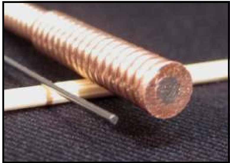
Cross sections of wires used for the highest and lowest note on the piano (balanced on a toothpick).
