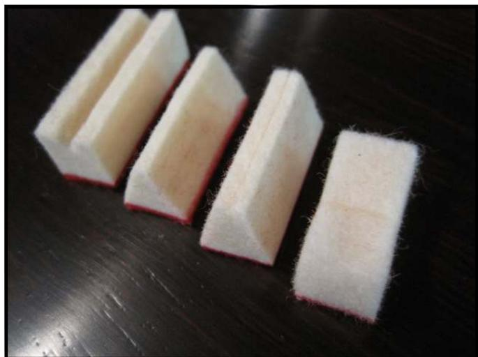
are shown single wedge dampers (used for the largest bass strings), double wedge dampers (used for notes with a pair of bass strings), trichord dampers (used for larger steel treble strings, and flat treble dampers (used for smaller steel treble strings). Obviously, a great deal of fine adjustment is necessary to make all these parts perform in unison with one another.
