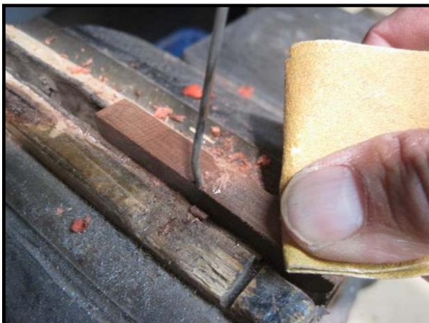
The lower surface of damper head is then scraped and sanded clean. The upper surface of the damper head may be cleaned and polished if the original lacquer finish is still in good shape. Otherwise, the old finish may need to be stripped off, so that a new lacquer finish can be applied (**note-extra work =extra cost**). A final step will be the polishing of the damper guide wires.
