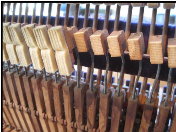
As the damper felts are removed, the damper blocks are returned to the same position they came from in the action.
