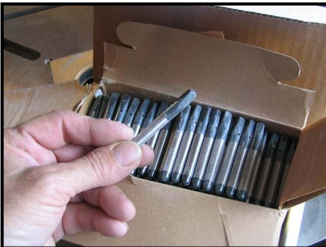
Tuning pins are a stock piano replacement part sold in sets. They are made from high-quality steel cut with micro-threads and are produced with extremely consistent diameter. Typically, the next size up from the factory set (which would be .004" larger) will be installed to give a tighter fit. Tuning pins do come in two finishes, blued (shown in photo) and nickle plated.
